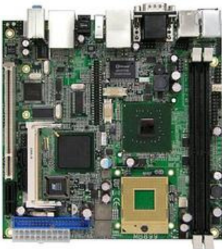
Figure 5 Sample small-factor Mini-ITX board (170mm x 170mm, 6.7" x 6.7")
